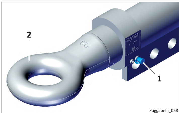
Figure 33: Location of grease nipple on BNA towing eye
