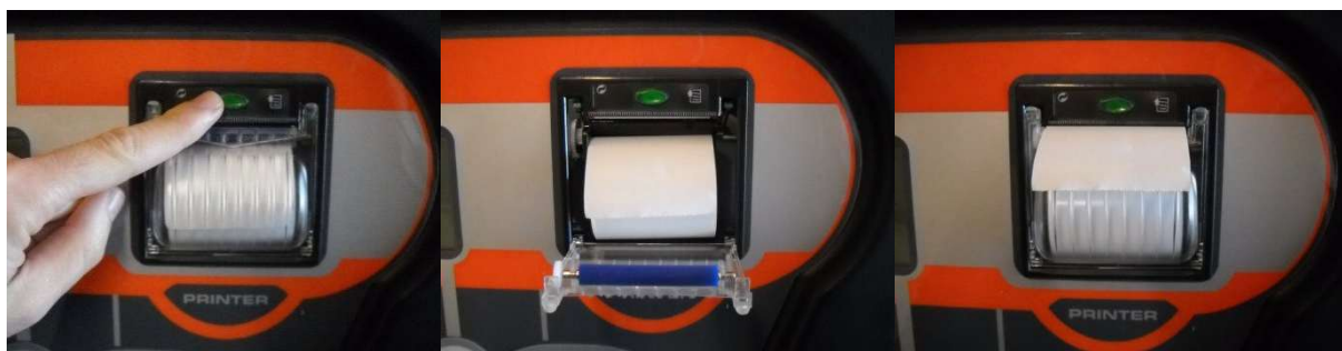
Image 8 – how to replace the paper
